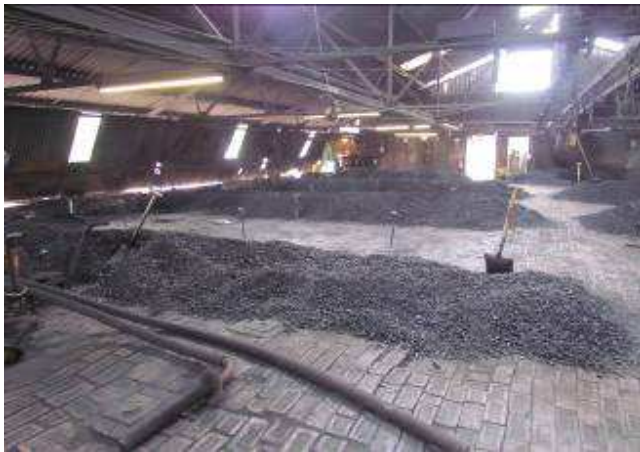
Coal drying on the floor (above the kiln)
